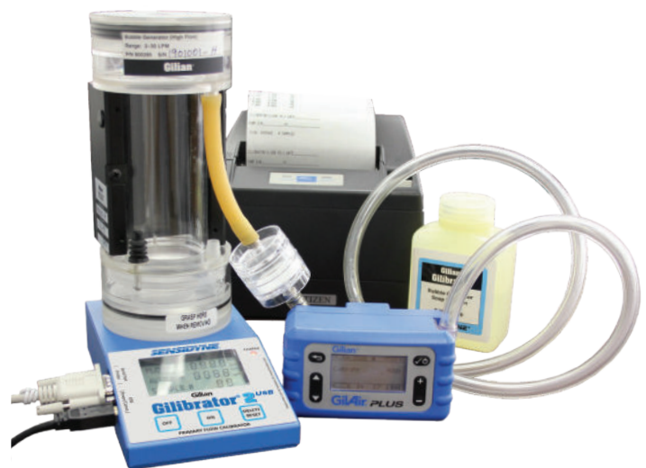
Gilibrator 2 USB shown calibrating the GilAir Plus air sampling pump, with optional Printer Kit and Bubble Soap Solution.
