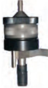
HD style cyclone with European style sampling cassette.
