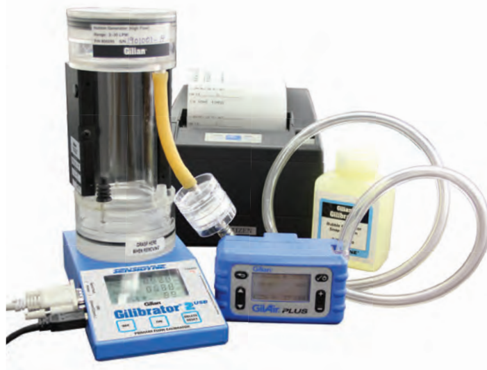
Gilibrator 2 USB shown calibrating the GilAir Plus air sampling pump, with optional Printer Kit and Bubble Soap Solution.
