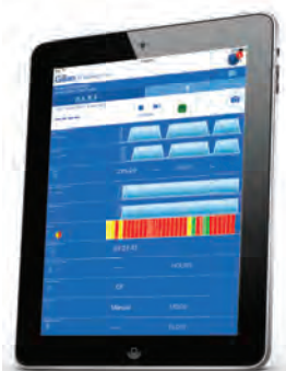
Sample data, as well as motion monitoring is available via Bluetooth connection to Android and iOS* devices running Gilian CONNECT Mobile.
