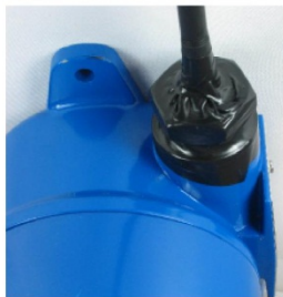
Figure 4-4 Water Proofing Antenna Connections
