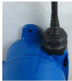
Figure 4-4 Water Proofing Antenna Connections
