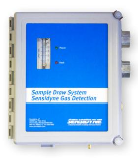
The Sensidyne Sample Draw System samples air from remote locations pulling a sample to gas detection transmitter(s) and is offered as a diaphragm pumped or an air operated aspirator unit. It is designed for placement in a Class I, Division 2 Hazardous (Classified) area to sample from a Class I, Division 1 Hazardous (Classified) area, Groups C and D. A Division 2 approval eliminates the need for flame arrestors and reduces related maintenance caused by dirt and moisture.
