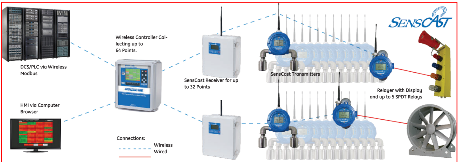
Drawing 2: Two independent networks consisting of a Receiver and 32 SensCast Transmitters (or 16 Dual Head Transmitters) exist in one facility. A Sensidyne wireless-enabled controller (Model 7200 shown) collects all 64 outputs sending them to a DCS or PLC via wireless Modbus. A SensCast Relayer actively “listens” for alarm or fault conditions and activates annunciators or hazard mitigation systems.
