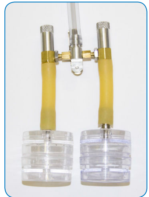
Top Access Model Shown with Two Filter Cassettes
